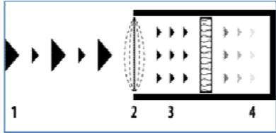
The acoustics of enclosed spaces is significantly affected by modal problems, below the Schroeder frequency. There are essentially only two known ways to minimize these resonances by absorption using either Helmholtz resonator designs or diaphragmatic membranes. RPG offers two types of low frequency membrane absorbers in its Modex line. The
