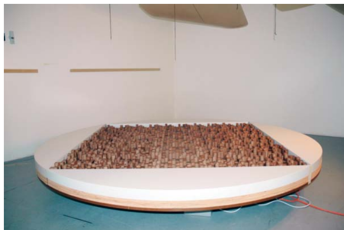
Figure 7.4. 1:1.5 sealed particle board Skyline on the rotating scattering coefficient table in the rev room for scattering coefficient testing.
