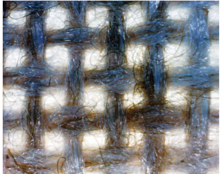
Figure 6.3. Image of a standard panel fabric at a magnification of 40X.
