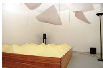
Figure 2.2 Absorption Coefficient ISO 354: How much of the incident sound is absorbed (Must be measured full scale).
