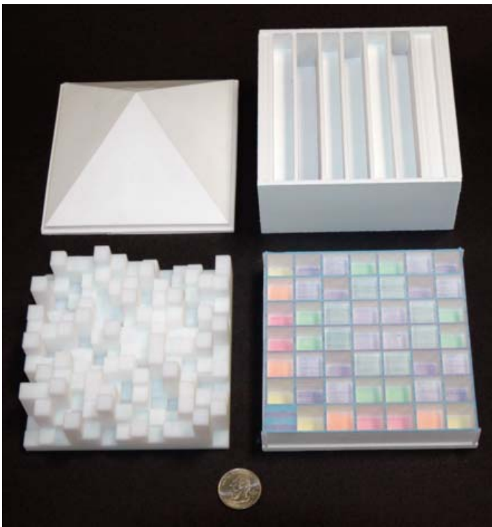
Figure 7.2. 1:5 scale model diffusors. Upper left: square based pyramid; Upper right: Modfusor; Lower left: Skyline; Lower right: Omnifusor. Coin in foreground is a US quarter.
