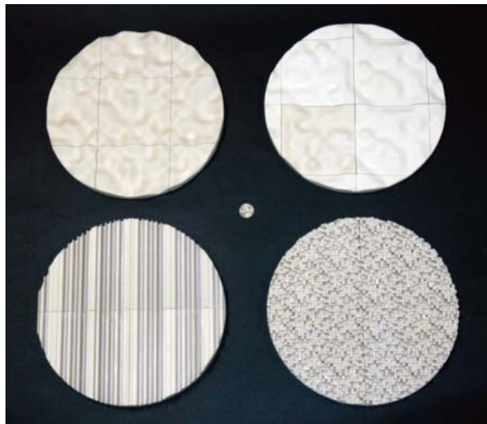
Figure 7.3. Four 1:10 scale samples for scattering coefficient testing according to ISO 17497-1. Upper left: Bicubic 8" deep; Upper right: Bicubic 4" deep; Lower left: Modfusor; Lower right: Skyline.
