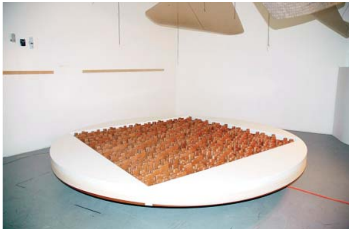
Figure 4.4. 1:1.5 Skyline on the rotating table in the rev room.
