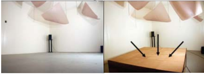
Figure 3.8. Top: Empty rev room showing diffusing clouds, loudspeaker and microphones. Bottom: Rev room with perforated wood panels in an E mount.
