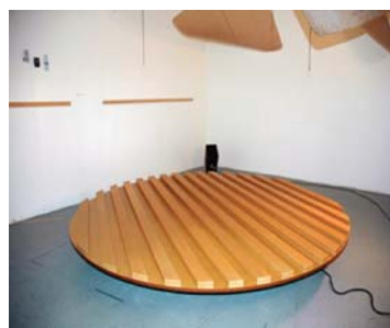
Figure 2.3 Scattering Coefficient ISO 17497-1: How much of the incident sound is scattered away from the specular zone (Can be measured in scale and calculated).
